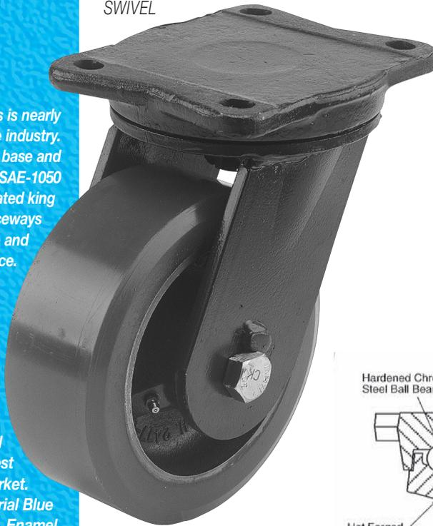
The ever-popular 110 series is nearly synonymous with the automotive industry. Hot forged top plate, yoke base and bearing retainer are made with SAE-1050 steel and features a strong integrated king pin with slotted adjusting nut. Raceways are flame hardened for longer life and better performance.
